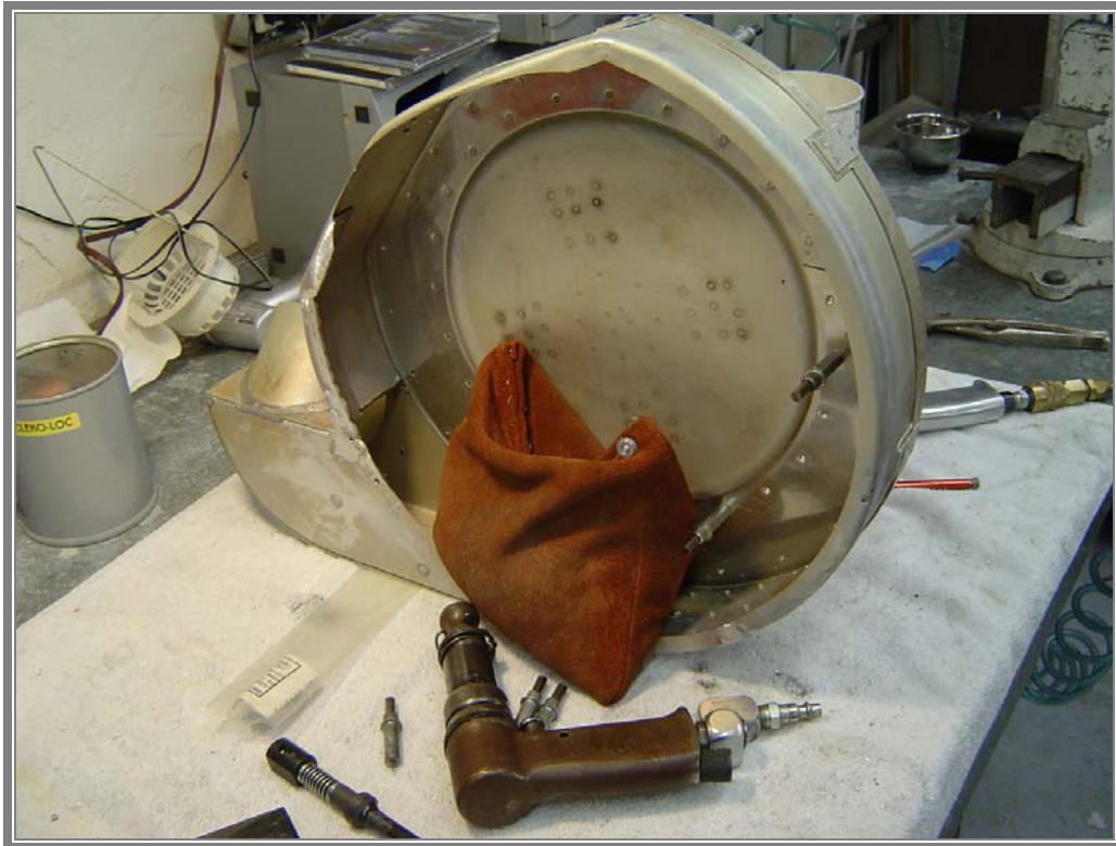
24568-000 BOX, TYPICAL REPAIR PROCESS
