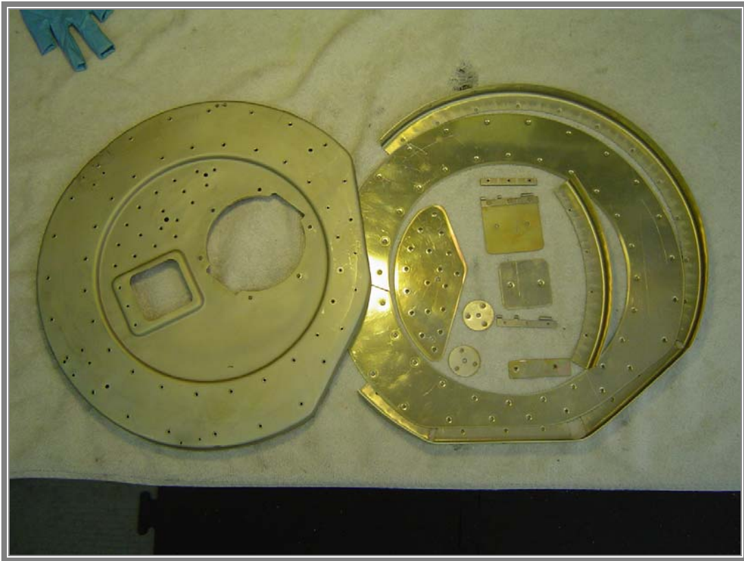
24569-000 PLATE, TYPICAL REPAIR COMPONENTS
