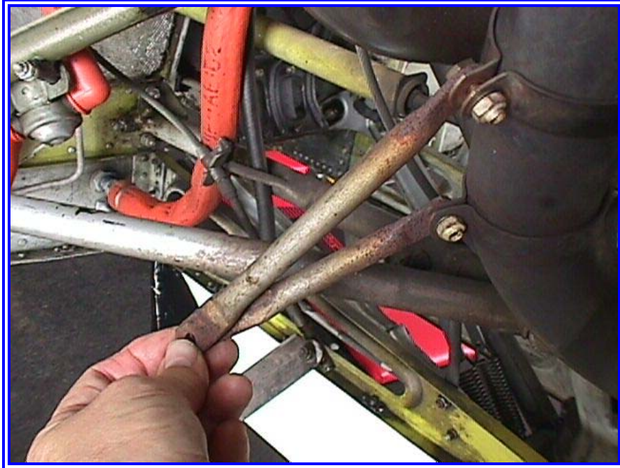
RIGHT SIDE MUFFLER SUPPORT TUBES AND CLAMPS POSITION
