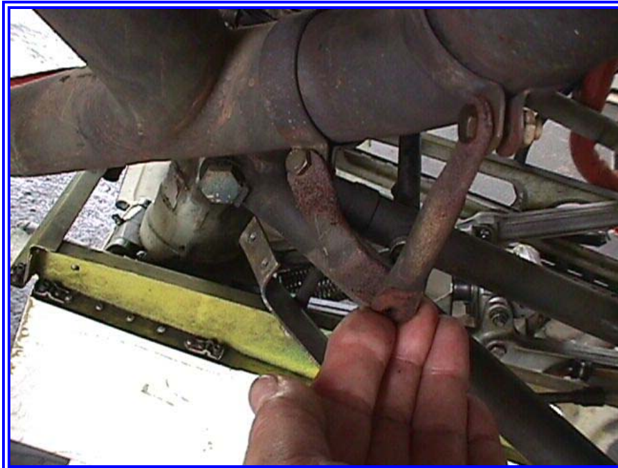
LEFT SIDE MUFFLER SUPPORT TUBES AND CLAMPS POSITION
