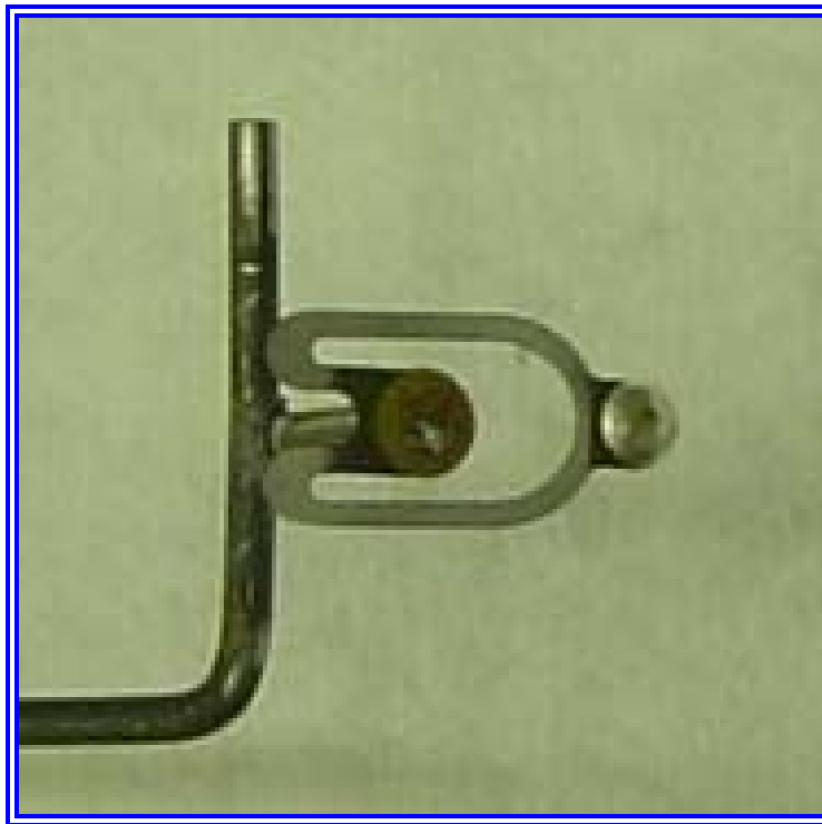
NOTE VERY SMALL WORN SPOT ON WIPER BUTTON, THIS IS OK; A LARGE WORN SPOT WOULD GIVE INACCURATE READINGS
