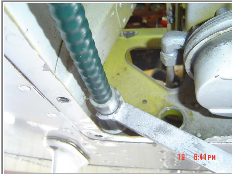
SPECIAL WRENCH USED TO TIGHTEN THE CASTLE NUTS. SEE MY NOTE ON PAGE ONE ABOUT EARLY SINGLE AIRFRAMES.
