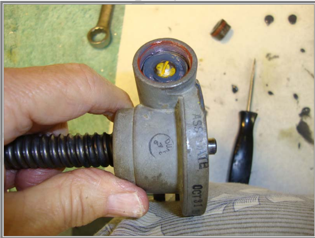
NEW BEARING AT DRIVE SHAFT.
