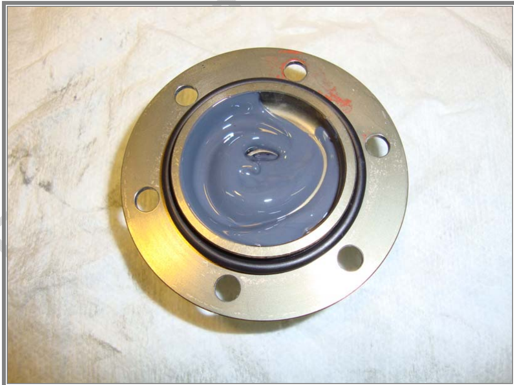
ENDPLATE WITH NEW O-RING AND DUKE'S SPECIAL LUBRICANT.
