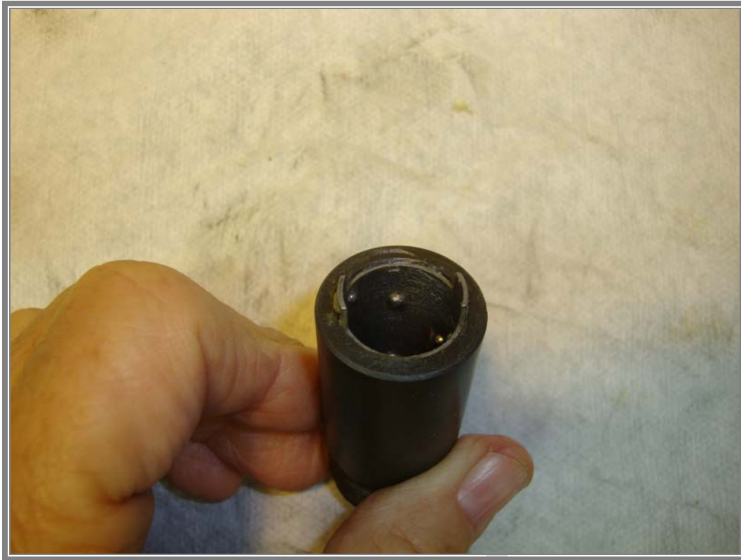
TRAVERSING NUT WITH NEW BALLS INSTALLED.
